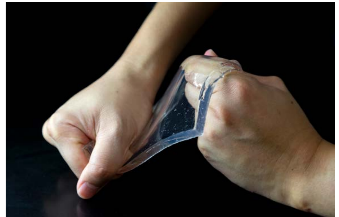
An ultra-tough double network gel (DN gel), which has a high breaking stress that offers the prospect of its application as a cartilage substitute, among other uses.
